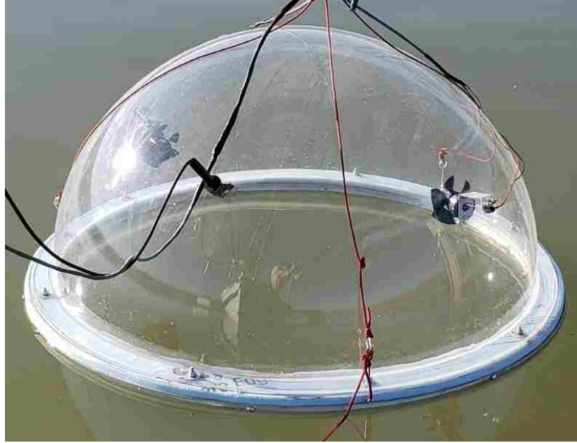
Figure 3.2: Hemispherical Evaporation Chamber (dome) during a validation test on September 30, 2018 on Cochiti Lake, New Mexico, USA.
